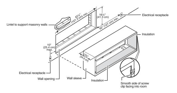
Note: All 230/208V units are manufactured with a 60" power cord. The receptacle locations above must be followed to ensure proper connections.
